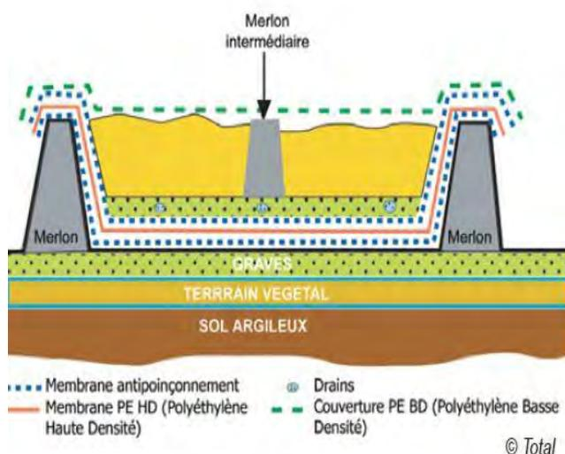
The graph on the left illustrates the applied waste storage facility of the Erika pollution incident as an example that could be applied to the Estancia oil spill.
