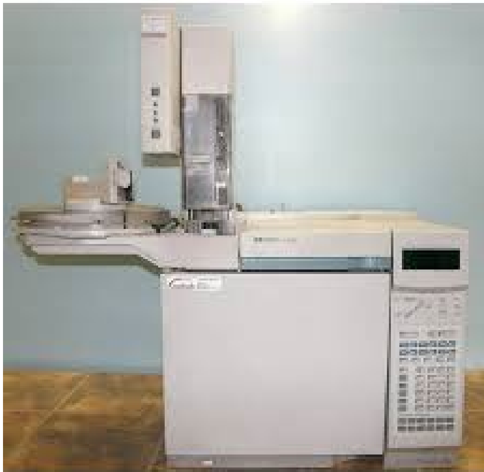
GC-FID used for EPH analysis
