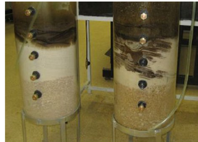
Fig. 1 Depth performance in dry sand (left) and dry carbonate (right) system
