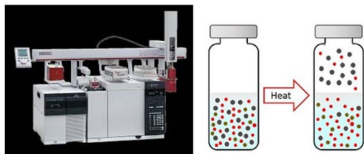
VOC analysis by Headspace GC-MS
