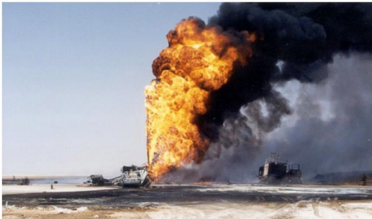
Oil well blow-out from sabotage causing spill directly onto land and air emissions
