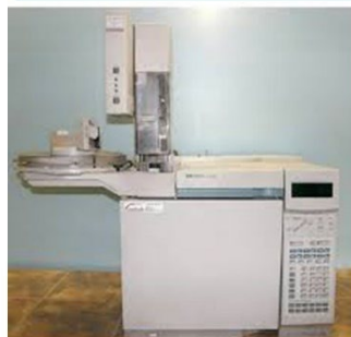
GC-FID used for EPH analysis
