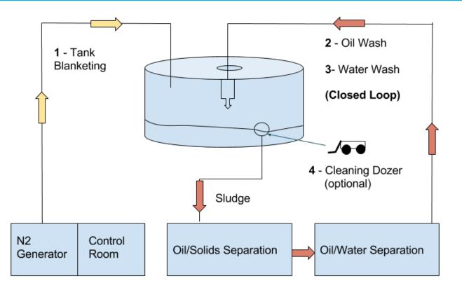
5 - Effluents: Oil, water, solids
